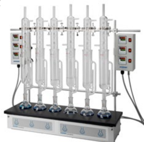
6-Place heating mantle with digital display controller
